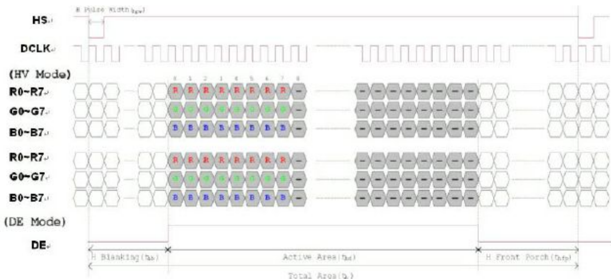
Figure 3. 1 Horizontal input timing diagram.
